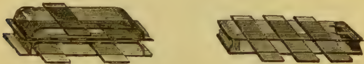
FIGS. 10, 11.—GLASS BENCHES FOR GLASS PLATES OR SLIDES.
